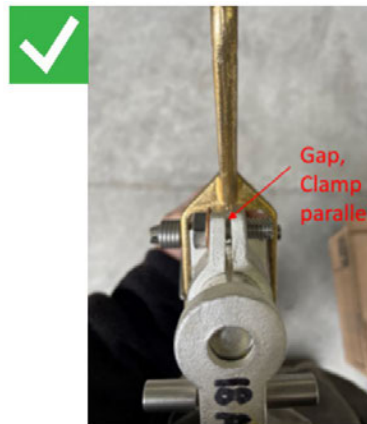
Figure 18 Proper End Fitting Installation
